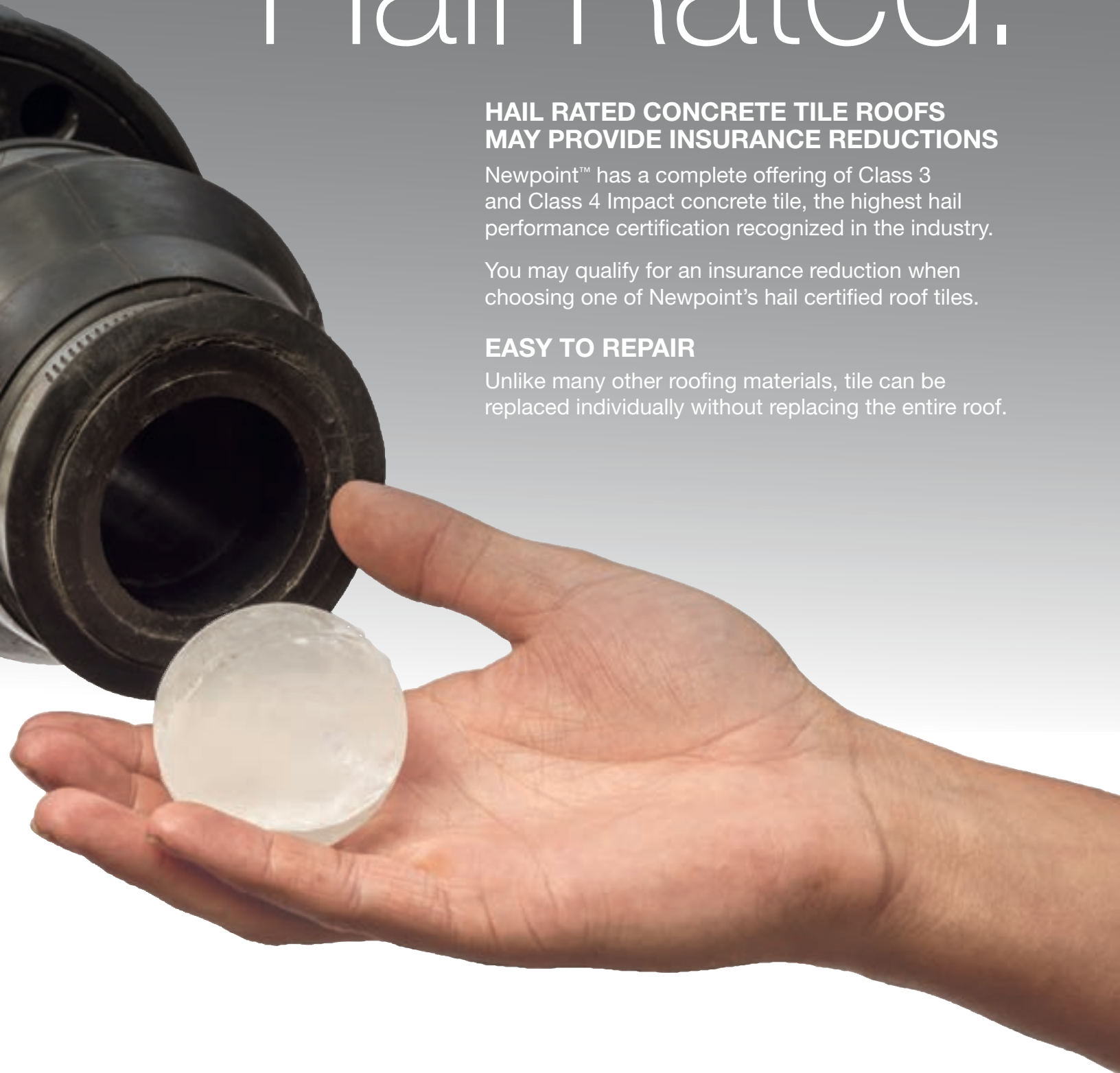
► The hail testing at Intertek's laboratory in Dallas, Texas under test protocol for FM 4473.
