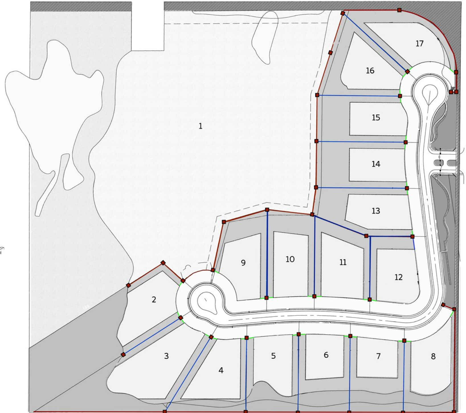
■ Required Fence Column Locations — Type A Fence only — Type A, B, B Alt, or Type D Fence — See Diagram for Street-Facing Fence Regulations
