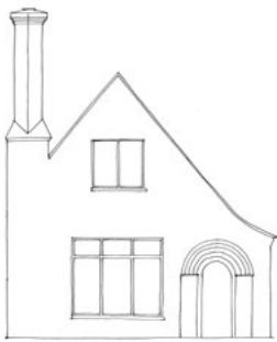
Swooped Asymmetrical Gable with Engaged Chimney
